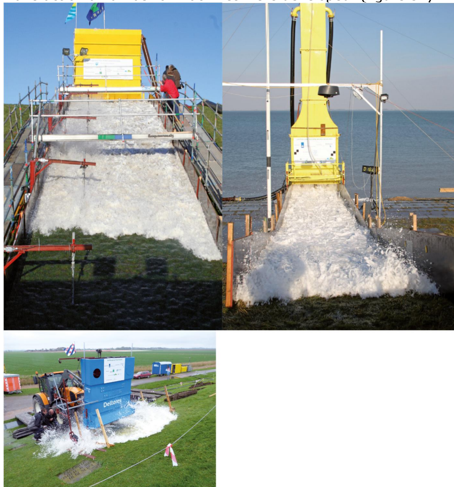
figure 31 Waveovertopping simulator, Wave runup simulator Waveimpact simulator [Van der Meer, 2014]
